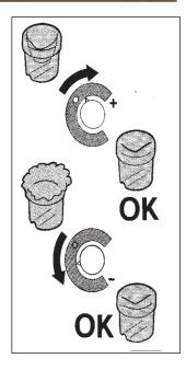
If it is thought necessary, the above situations can be rectified by, in the first case, turning the control knob (as little or as much as is required) clockwise and, in the second case, turning the knob to the right counterclockwise.
